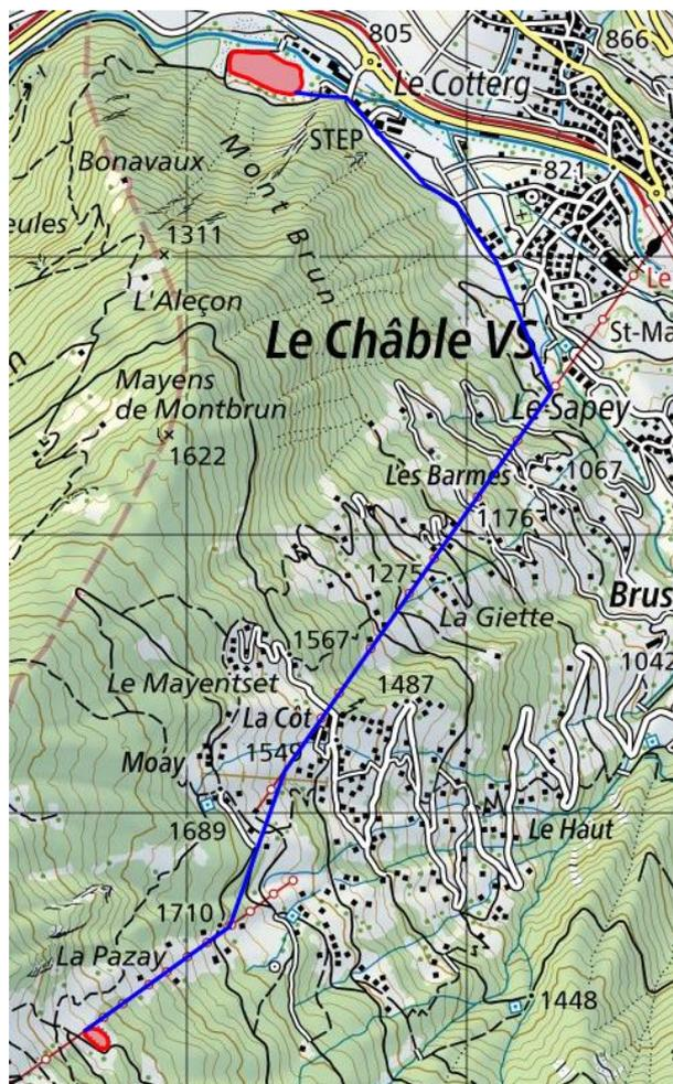
Figure 4: Geographical location of the Moneyeu - Vernays reservoirs (red surfaces). The preliminary piping path connecting the two reservoirs is shown by the blue line. Source: Swisstopo
